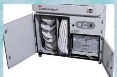
**Integrated Extraction/Filtration** Filters debris and fumes from the laser, returning safe clean air to the room. Incorporates large capacity pre filter(s), HEPA filter and 40L activated carbon filter (refillable on LS100 & LS100Ex). Simple to fit replacement/spare filters available.
