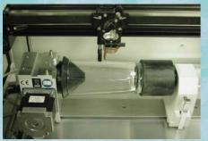
Rotary Attachment Removable device to facilitate the engraving of cylindrical objects. Supplied with a variety of concave and convex cones to grip multiple component shapes and sizes.
