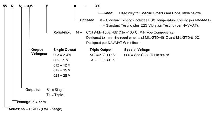
**Example:** 55KT1-515M1 = DC/DC (Low Voltage); 75 Watt; Triple Output; 5 V, ±15 V; COTS-Mil-Type; ESS Vibration Testing
