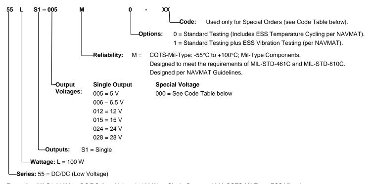
**Example:** 55LS1-012M1 = DC/DC (Low Voltage); 100 Watt; Single Output; +12 V; COTS-Mil-Type; ESS Vibration
