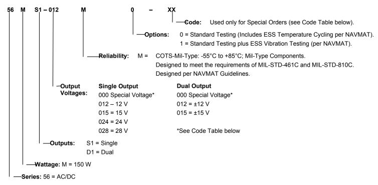
Example: 56MD1-012M1 = AC/DC; 150 Watt; Dual Output; ±12 V; COTS-Mil-Type; ESS Vibration Testing
