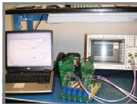
Characterization of 5-slot ATCA backplane using Elma Bustronic's unique probe card
