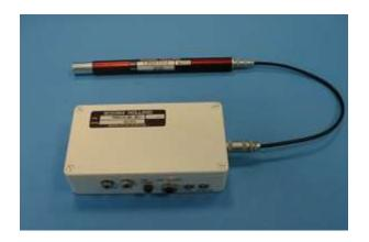
The signal and power supply junction box provides the high voltage to the probe and processes the analog signal from the PMT.
