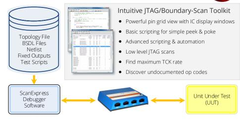
ScanExpress Debugger uses a simple JTAG interface with multiple tools to control and observe signals on the UUT
