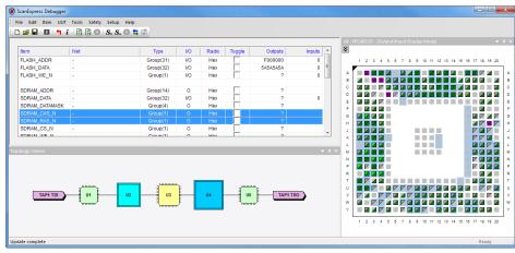
The ScanExpress Debugger Grid View and display windows allow convenient control and observation of all boundary-scan signals in a system
