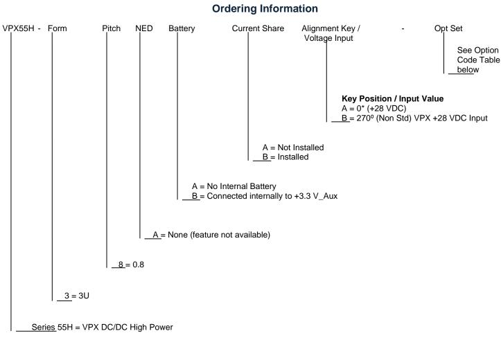
**Example:** VPX55H-38AABA-00 = 3U VPX DC/DC Converter; 0.8" pitch; no NED feature; no internal battery; current share on VS1, VS2, and VS3; +28 VDC innput; 500-Watt output power
