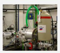
36 pixel detector for EXAFS at Soleil Synchrotron
